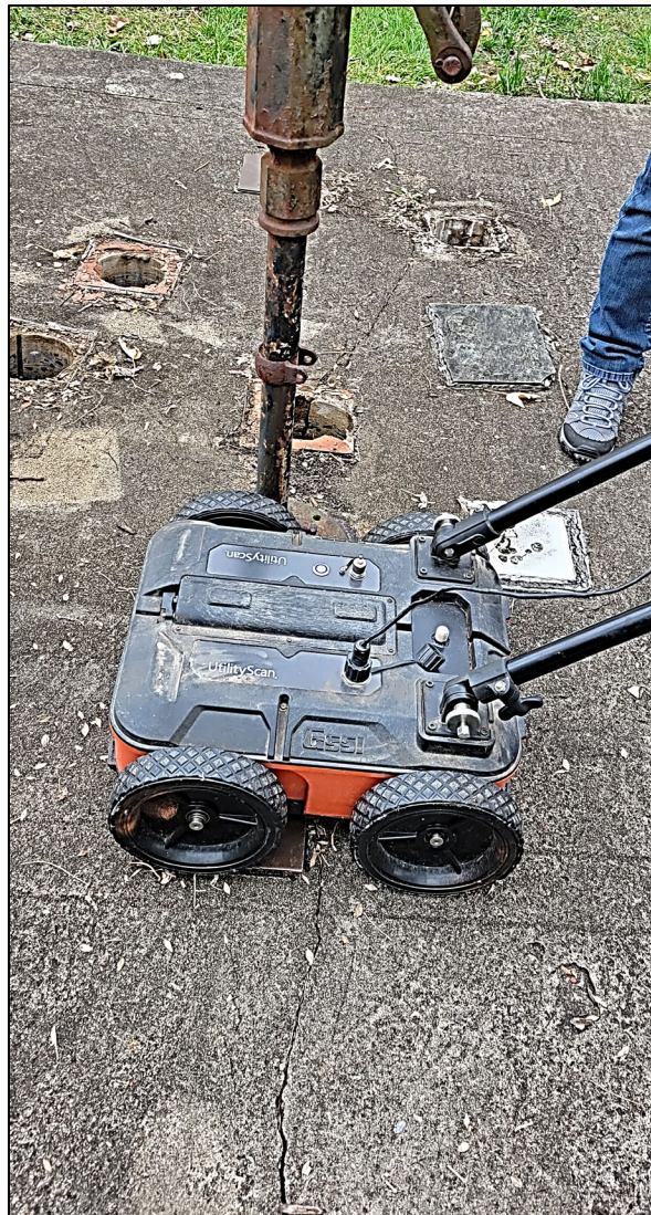
Figure 4: Photograph image of a portion of the Ft. Loudoun concrete Well Cap. Seven (7) covered and open bore holes in the concrete slab are visible. Note the two (2) parallel lines inscribed into the concrete Well Cap. A Geophysical Survey Systems, Inc., (GSSI) UtilityScan-B System with a Hyperstacking 350MHz antenna, integrated cart, and RADAN 7 Software for data processing is also shown in the image. It was used in the Ground Penetrating Radar (GPR) Survey of the extant c. 103' Ft. Loudoun Well and the area immediately around the Well Cap, Area #1. Photograph by Mark Michael Ludlow RPA, October 2023.
