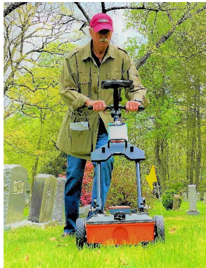
Figure 2: Photographic image (Not from the Ft. Loudoun GPR Survey) of the Geophysical Survey Systems, Inc., (GSSI) UtilityScan-B System with a Hyperstacking 350MHz antenna, integrated cart, and RADAN 7 Software for data processing, used in the Ft. Loudoun Open Spaced Ground Penetrating Radar (GPR) Survey. The individual in the image is the Ft. Loudoun GPR Survey Principal Investigator. Photograph by Lucy Goddin, Former Executive Director of the historic Ivy Hill Cemetery in Alexandria, Virginia, 2016.
