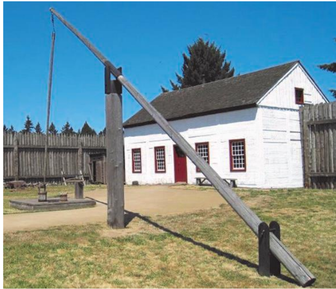
Figure 4 Well Sweep at Fort Vancouver Photo courtesy of U.S. National Park Service
